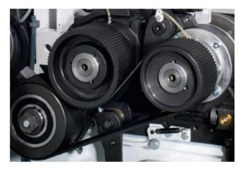
**High-capacity grinding** The compact roll pack with self-contained forces ensures a high setting accuracy and grinding stability. The low-maintenance toothed gear transmission guarantees smooth running.
