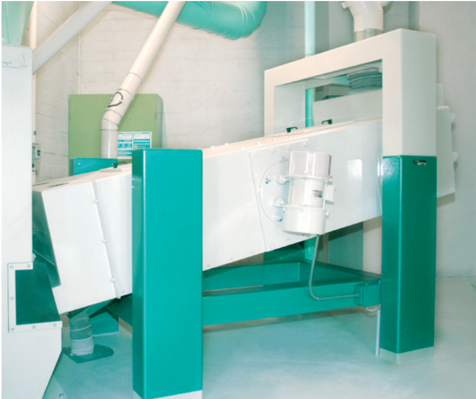
Separator MTRB with aspiration channel MVSH.
